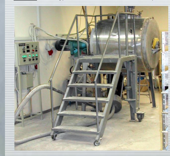
Capacity: 100 kg/charge **Reactor volume**: 0.45 m<sup>3</sup> Vacuum pump, condenser Spraying: pneumatic nozzle Mixing: horizontal impeller Heating: electric heating mantel with temperature control During the drying and heat treatment the temperature is changing continuously. The reaction can take place in the drying period too.
